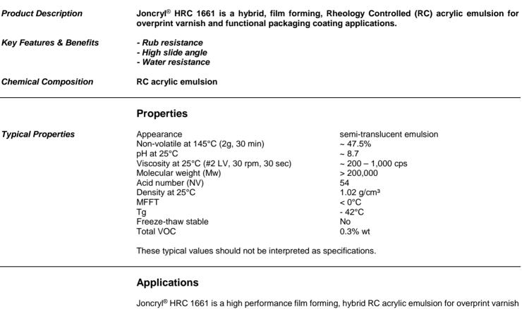
Joncryl<sup>®</sup> HRC 1661 is a high performance film forming, hybrid RC acrylic emulsion for overprint varnish applications. It provides significant improvements in rub and water resistance at a cost equal to comparable acrylic emulsions. It can be used as a letdown vehicle in paper and paperboard inks. The flexibility of Joncryl<sup>®</sup> HRC 1661 will enhance the rub resistance of inks even when used at low levels.
