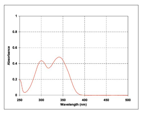
Tinuvin<sup>®</sup> 329 exhibits strong absorbance in the 300 – 400 nm region and minimal absorbance in the visible region (> 400 nm) of the spectrum. The absorption maxima are at 301 nm and 343 nm ( $\epsilon$  = 15910 l/mol·cm) in chloroform solution.
