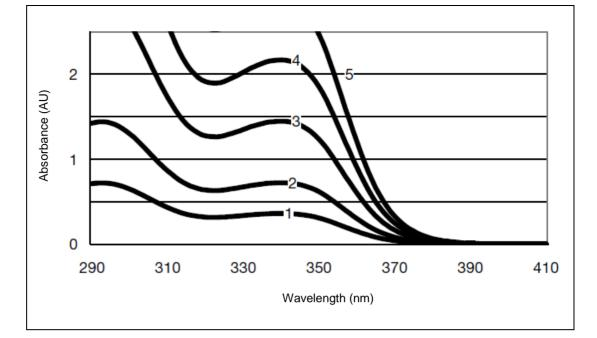
**UV Transmission Spectrum** (The theoretical concentration of the UVA in an applied 40 µm clear coat was calculated as a function of the concentration in toluene with the help of the Lambert-Beer law. Spectra were recorded in toluene, light path length = 1 cm.)
