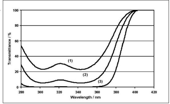
Line one: 0.003 % Tinuvin® 5060 corresponds to 0.38% active UVA in a 40  $\mu$ m film Line two: 0.005 % Tinuvin® 5060 corresponds to 1.35% active UVA in a 40  $\mu$ m film Line three: 0.014 % Tinuvin® 5060 corresponds to 3.38% active UVA in a 40  $\mu$ m film
