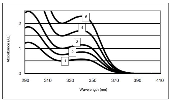
UV Transmission Spectrum (The theoretical concentration in an applied 40 µm clear coat was calculated as a function of the concentration in toluene with the help of the Lambert-Beer law. Spectra recorded in toluene, light path length = 1 cm)
