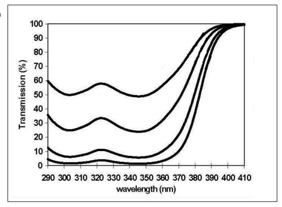
Top Line: 0.001% Tinuvin® 99, corresponds to 0.25% in a 40  $\mu$ m film Second Line: 0.002% Tinuvin® 99, corresponds to 0.50% in a 40  $\mu$ m film Third Line: 0.004% Tinuvin® 99, corresponds to 1.0% in a 40  $\mu$ m film Bottom Line: 0.006% Tinuvin® 99, corresponds to 1.5% in a 40  $\mu$ m film
