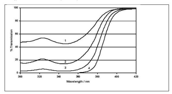
Line one: 0.0025 % Tinuvin® 9945-DW (N) corresponds to 0.30 % active UVA in a 40  $\mu$ m film Line two: 0.005 % Tinuvin® 9945-DW (N) corresponds to 0.60 % active UVA in a 40  $\mu$ m film Line three: 0.010 % Tinuvin® 9945-DW (N) corresponds to 1.20 % active UVA in a 40  $\mu$ m film Line four: 0.020 % Tinuvin® 9945-DW (N) corresponds to 2.40 % active UVA in a 40  $\mu$ m film
