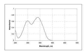
Tinuvin P exhibits strong absorbance in the 300-400 nm region and minimal absorbance in the visible region (>400 nm) of the spectrum. The absorption maxima are at 301 nm and 341 nm ( $\varepsilon=16'150$  l/  $mol\cdot cm$ ) in chloroform solution
