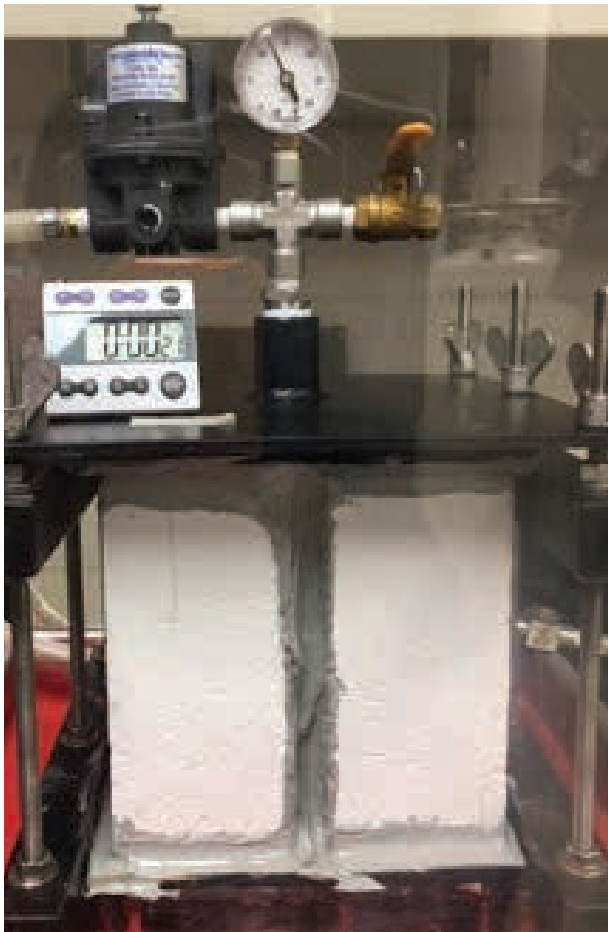
Top left: ASTM D 7088 test set up to evaluate waterproofing coatings under hydrostatic pressure.
