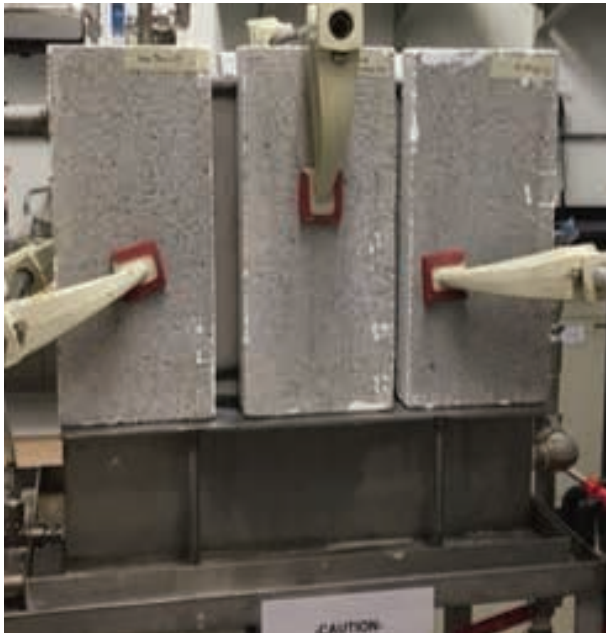
Top left: ASTM D 6904 test apparatus to evaluate waterproofing coatings under wind-driven rain. The coated side of the blocks are facing the inside of the apparatus (i.e., not visible).
