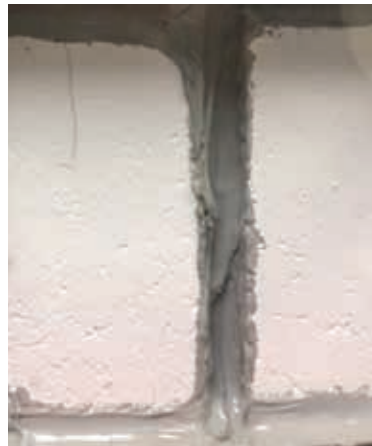
Top right: Performance of coating formulated with Acronal 4160 passing ASTM D 7088 without blistering or coating failure.
