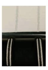
**Left:** ASTM D711 test set up to evaluate dry no-pick-up time of traffic paint coatings. Formulations with ACRONAL Xpress 4347 (bottom) and formulations with competitive latex A (top) both exhibit no-pick-up at four minutes and 30 seconds.
