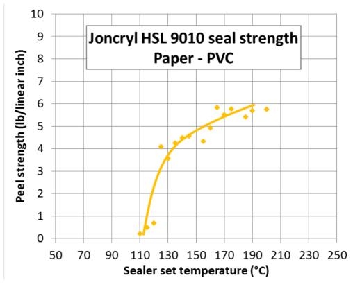
The plot above shows the bond strength at various sealing temperatures. The Joncryl HSL 9010 was applied neat, with a wire wound bar, to 18 pt SBS paper stock and 1mm PVC sheet. The coated surfaces are sealed together at 1 bar/14.5 psi for 1 second. Results will vary with substrate thickness, seal pressure and seal time.
