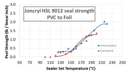
The plot above shows the bond strength at various sealing temperatures. The "Unformulated" curve shows Joncryl HSL 9012 applied neat, while the "Formulated" curve was generated with the starting point formula below. Coatings were applied with a wire wound bar to 2.5 mm O-temper aluminum foil and sealed to 1mm PVC sheet. The coated surfaces are sealed together at 1 bar/14.5 psi for 1 second. Results will vary with substrate thickness, seal pressure and seal time.
