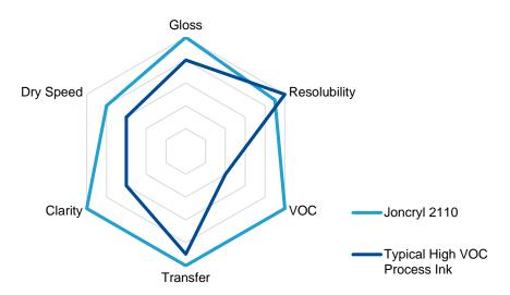
Joncryl 2110 Improved transfer vs. Typical High VOC Process Ink
