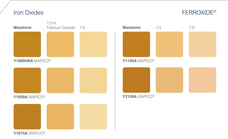
With clean shades and low oil absorption, this range of permanent, non-bleeding pigments can either be used alone or in combination with organic pigments to improve opacity, reduce formula cost and add UV resistance to coating and ink formulations. MAPICO® Yellows will suit a range of applications including coatings, colorants, paper, adhesives and stucco. All grades are micronized and offer easy dispersion. MAPICO® Y1000HRA has improved heat stability.
