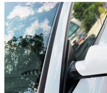
WINDSHIELD WATER GUIDE TRIM, SEBS COMPOUND ON PP CORE IN INJECTION MOLDING PROCESS
