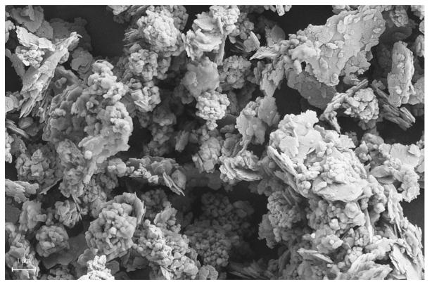
Classic Neuburg Siliceous Earth is a natural combination of corpuscular, cryptocristalline and amorphous silica and lamellar kaolinite: a loose mixture impossible to separate by physical methods. As a result of natural aging, the silica portion exhibits a round grain shape and consists of aggregated cryptocristalline primary particles of about 200 nm diameter which are coated partially opallike. This unique structure leads to good application properties.
