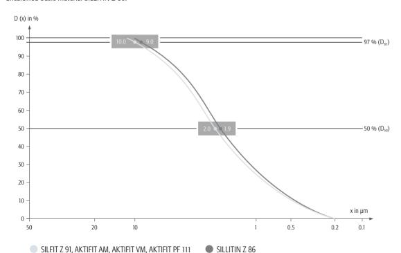
The measuring method for this particle size distribution is based on the Fraunhofer analysis of diffraction spectra. The analyses were performed with the Mastersizer 3000, a laser device from Malvern Instruments.
