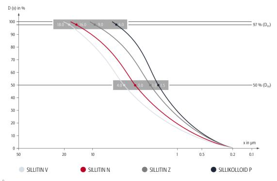
The measuring method for this particle size distribution is based on the Fraunhofer analysis of diffraction spectra. The analysis were performed with the Mastersizer 3000, a laser device from Malvern Instruments.
