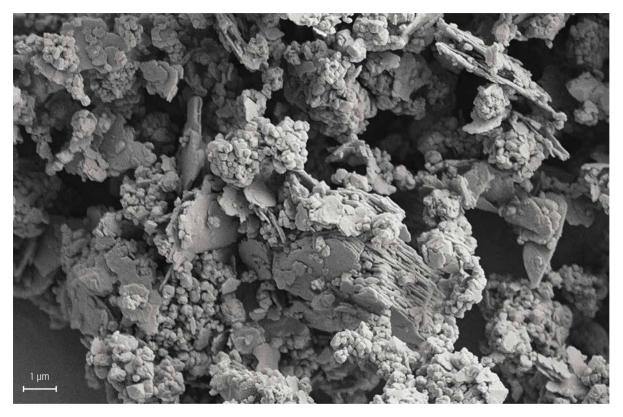
Our calcined products SILFIT and AKTIFIT are based on the standard product SILLITIN Z 86. A thermal process is used to expel the crystalline water in the kaolinite portion and new mineral phases are formed practically amorphous. The silica portion remains inert at the temperature used. The resulting products have an outstandingly high degree of white and color neutrality.
