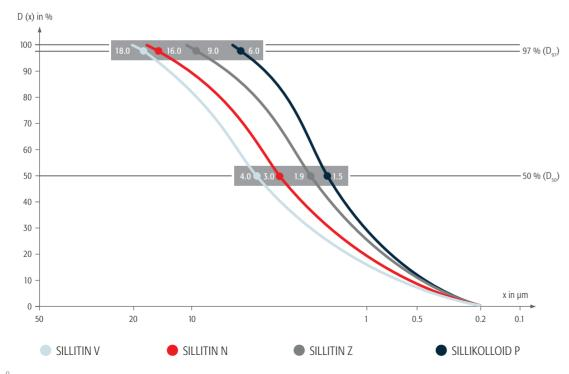
The measuring method for this particle size distribution is based on the Fraunhofer analysis of diffraction spectra. The analyses were performed with the Mastersizer 3000, a laser device from Malvern Instruments.
