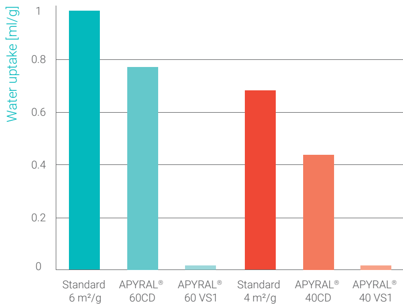
Water uptake of ATH / APYRAL® powder according to Baumann values of saturation after 30 min
