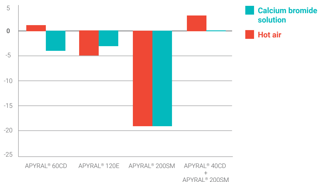
Change [%] of elongation at break after ageing (100 °C / 7 days – 135 °C / 7 days), EVM 600-compounds, 160 phr APYRAL ®
