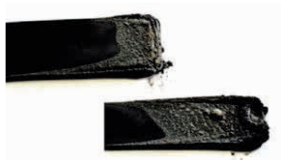
Specimen of glass fibre reinforced PA 6 (GF: 22.5 wt.-%) filled with DEPAL (13.5 wt.-%) and ACTILOX® 200SM (5 wt.-%) passes UL94 V0 at 0.8 mm.
