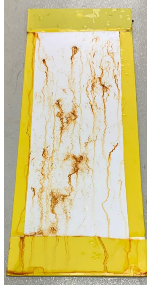
Joncryl PRO 1522 on Steel for 412 hours
