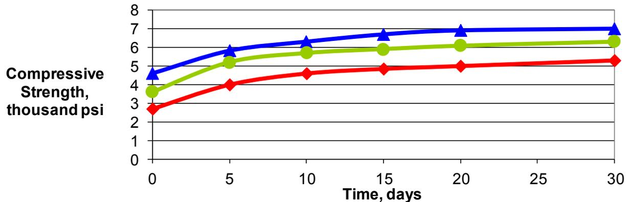
The chart above shows **Lomar<sup>®</sup> D Powder** at levels of 0.36% and 0.66% produced 18% and 25% water reduction respectively in Type 1 Cement and achieved higher compressive strength values than the control.
