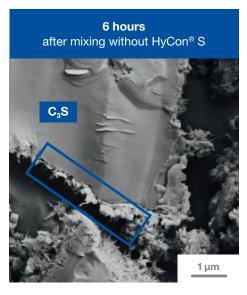
Small amounts of C-S-H are formed at the surface of C<sub>3</sub>S (blue rectangle)
