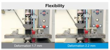
Improved flexibility due to reduction of E module allows appropriate RDP content reduction
