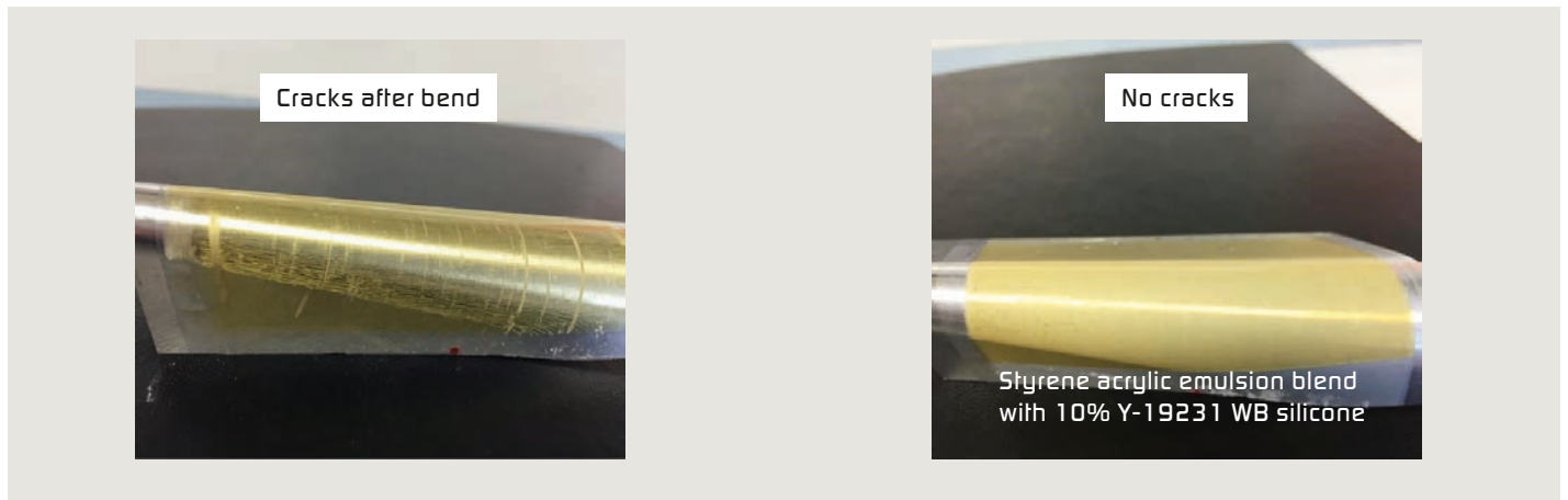
Figure 1: Improvement in flexibility (mandrel bend test) with the addition of silicone emulsion.
