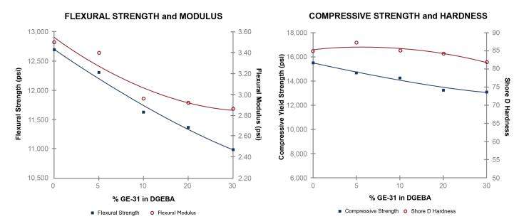
The effect of ERISYS<sup>®</sup> GE-31 on the cured properties of liquid epoxy resin (EEW 188) cured with TETA, cont.
