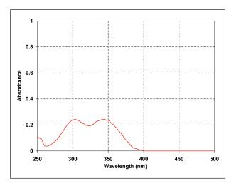
Tinuvin 213 exhibits strong absorbance in the 300-400 nm region and minimal absorption in the visible region (>400 nm) of the spectrum. The absorption maxima are at 303 nm and 344 nm ( $\varepsilon$  = 15'710 l/ mol·cm) in chloroform solution.
