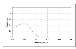
Tinuvin 312 exhibits strong absorbance in the 250–350 nm region and no absorbance in the visible region (> 400 nm) of the spectrum. The absorption maximum is at 305 nm in chloroform solution.
