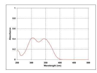
Tinuvin 328 exhibits high absor-bance in the 300-400 nm region and minimal absorbance in the visible region (>400 nm) of the spectrum. The absorption maxima are at 306 nm and 347 nm ( $\varepsilon$  =14'760 l/mol·cm) in chloroform solution.
